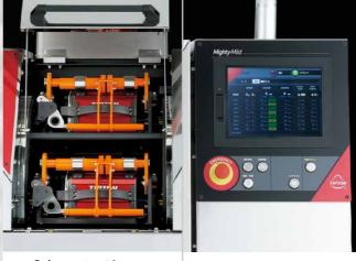
Color contrast for easy recognition to confirm mounting of barrels without fail
