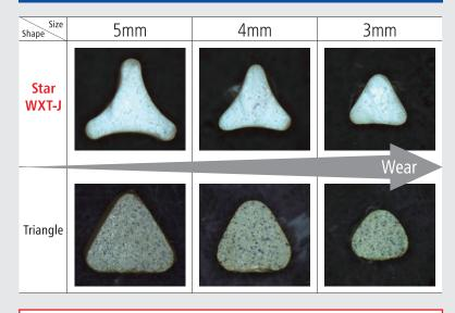
Star media can maintain its star shape while wearing to ensure proper contact with gaps
