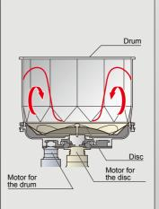
The centrifugal force of high RPM spinning disc forces particles into the sides then the inner wall of the drum forces the particles up.
