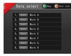
Up to eight operation conditions can be registered. Even if there are many types of workpieces, detailed operation settings for each type can be recalled easily. This prevents defective processing due to incorrect settings.
