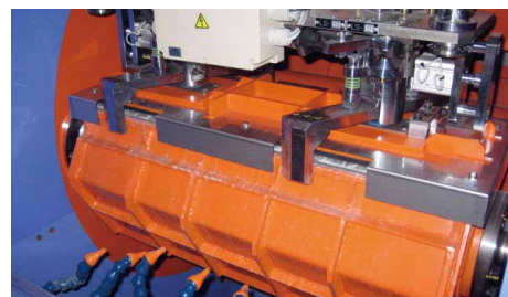
蓋の開閉機構／Structure of Opening and Closing of Barrel Lid
