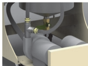
Slurry Pump and Polyurethane Joint
