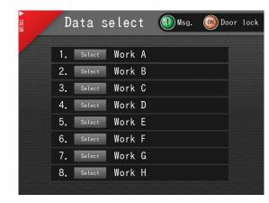
Up to eight operation conditions can be registered. Even if there are many types of workpieces, detailed operation settings for each type can be recalled easily. This prevents defective processing due to incorrect settings.
