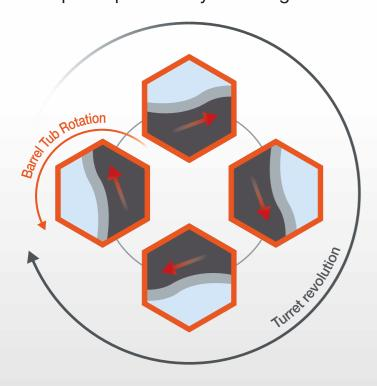
Barrel tubs with a hexagonal cross-section are placed on a rotating turret. Each barrel tub rotates on its axis in the opposite direction to the turret rotation (revolution). This planetary rotation motion allows the workpiece to slide on the mass surface and be polished.
