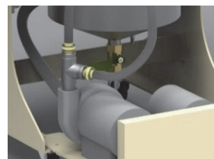
Slurry Pump and Polyurethane Joint
